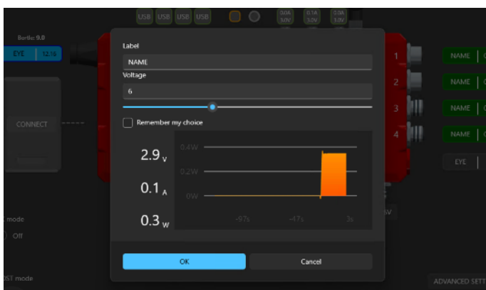
Image 46: advanced options window of one of the 3-12V power out ports
